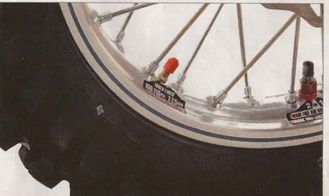
We had great results with the new TUBliss tubes. They allow you to run low air pressure without the fear of flatting or spinning the tire on the rim. Slavens swears by them!
