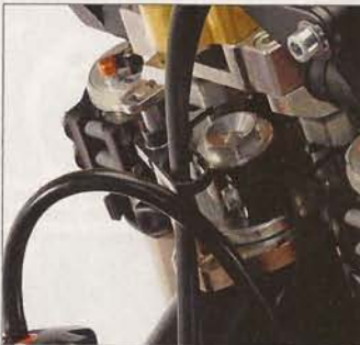
Hooked to the Scotts mount is a fancy machined-aluminum throttle cable guide. It keeps the throttle cables away from the stabilizer, handlebar clamp and handlebars, preventing wear and potentially dangerous cable snags. It sells for $19.95. Fork button speed bleeders ($36.95) are key for quick bleeds, and the billet star compression adjusters ($24.95) are stronger and more ergo-friendly than the stockers.
