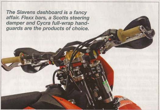
Hooked to the Scotts mount is a fancy machined-aluminum throttle cable guide. It keeps the throttle cables away from the stabilizer, handlebar clamp and handlebars, preventing wear and potentially dangerous cable snags. It sells for $19.95. Fork button speed bleeders ($36.95) are key for quick bleeds, and the billet star compression adjusters ($24.95) are stronger and more ergo-friendly than the stockers.
