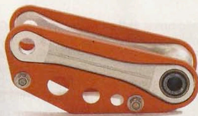
Slavens is working on a guard for the low-hanging linkage.
